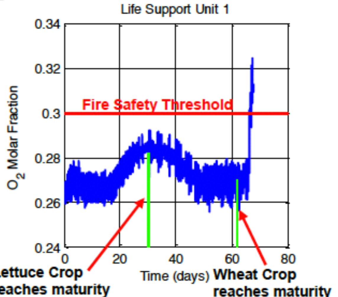
Fig. 9: Life Support Unit O<sub>2</sub> Molar Fraction
